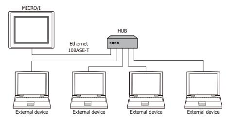
Up to 4 external devices can communicate with a single MICRO/I unit at one time.
