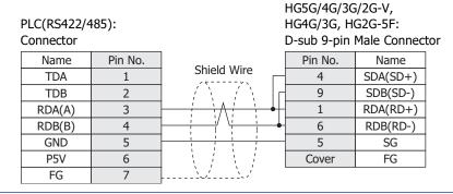
• When connecting COM1 on the HG5G/4G/3G/2G-V, HG4G/3G, HG2G-5F to the external device, do not insert terminating resistor to the external device. If terminating resistor can not be removed, use COM2 on the HG5G/4G/3G/2G-V, HG4G/3G, HG2G-5F instead of COM1.
