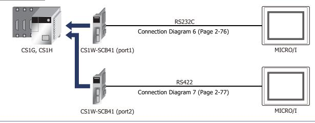
You can use the same cable for Connection Diagram 6 as for Connection Diagram 5.
