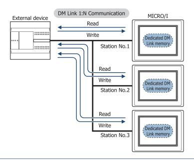
The Event Transmission function cannot be used with DM Link 1:N Communication.
