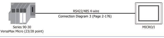
Connects to Serial port on Series 90-30 PLC Power Supply. Connects to Serial port 2 on VersaMax Micro PLC.
