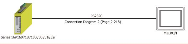
A touch-panel connection module is needed for Series 16i, 160i, 18i, 180i, 30i, 31i, 32i. For details, please contact FANUC LTD.
