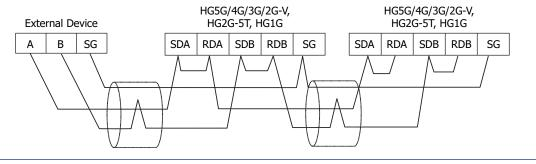
If more than one MICRO/I is connected to an external device, select **RS422/485 2-wire** from **Serial Interface** under **Interface Settings**.
