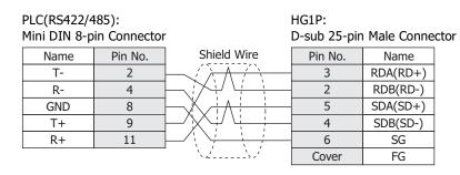
• Connection Diagram 4: S7-300 MPI Interface (RS485)
