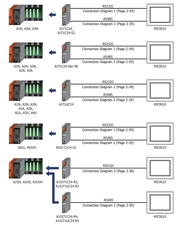
• MELSEC-A Series (Connects to CPU Module Link Interface)
