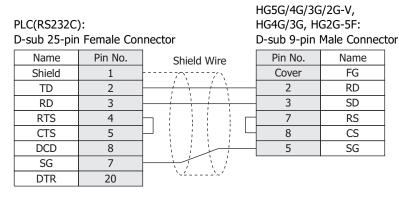
PLC(RS232C): D-sub 25-pin Female Connector
