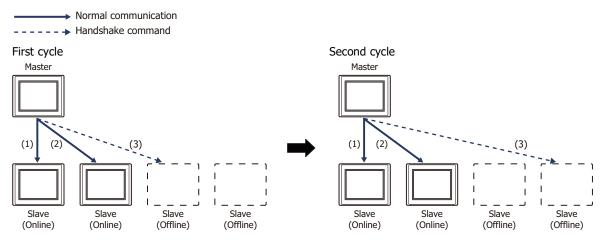
The Time Out duration for the command that detects the presence/absence of a slave (hereafter referred to as a handshake command) is set to 30 msec on the master.
