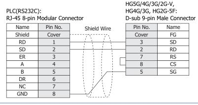
In case of the HG5G/4G/3G/2G-V, HG4G/3G, HG2G-5F a communication cable (Type Number: FC6A-KC2C) is available. Refer to Chapter 7 "1.6 User Communication or PLC communication cable (Type Number: FC6A-KC2C)" on page 7-5 about the connection diagram of the FC6A-KC2C.
