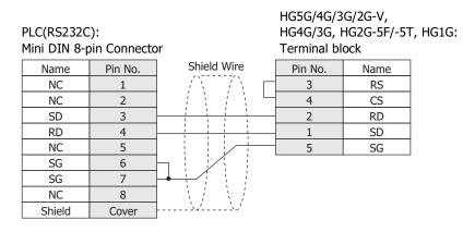
In case of the HG5G/4G/3G/2G-V, HG4G/3G, HG2G-5F/-5T, HG1G a communication cable (Type Number: FC2A-KP1C, HG9Z-XC275) is available. Refer to Chapter 7 "1.1 User Communication, Printer or PLC communication cable (Type Number: FC2A-KP1C, HG9Z-XC275)" on page 7-1 about the connection diagram of these cables.
