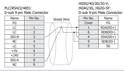
It is also possible to connect multiple PLCs and multiple MICRO/Is on the same network. Short-circuit the RDA and SDA of MICRO/I, and then connect to SIG-B of PLC. Short-circuit the RDB and SDB of MICRO/I, and then connect to SIG-A of PLC. Refer to S7-200 manual for restrictions when using multi-drops. When using multiple PLCs to communicate to multiple MICRO/Is, it will take extra time to establish communication between PLCs and OIs.
