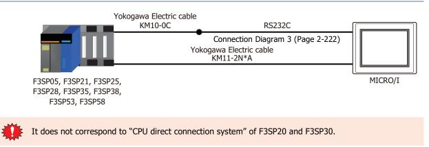
It connects with the port for programming tools of a CPU unit.
