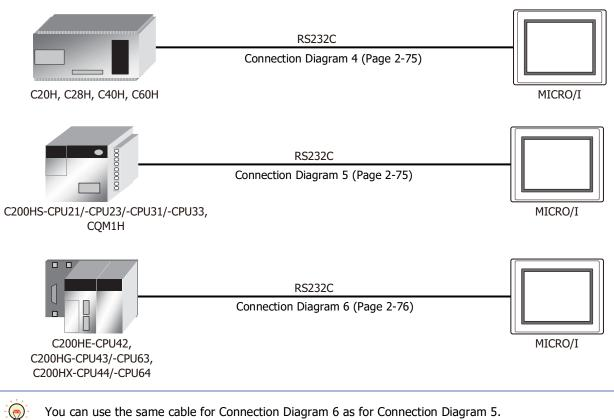
You can use the same cable for Connection Diagram 6 as for Connection Diagram 5.
