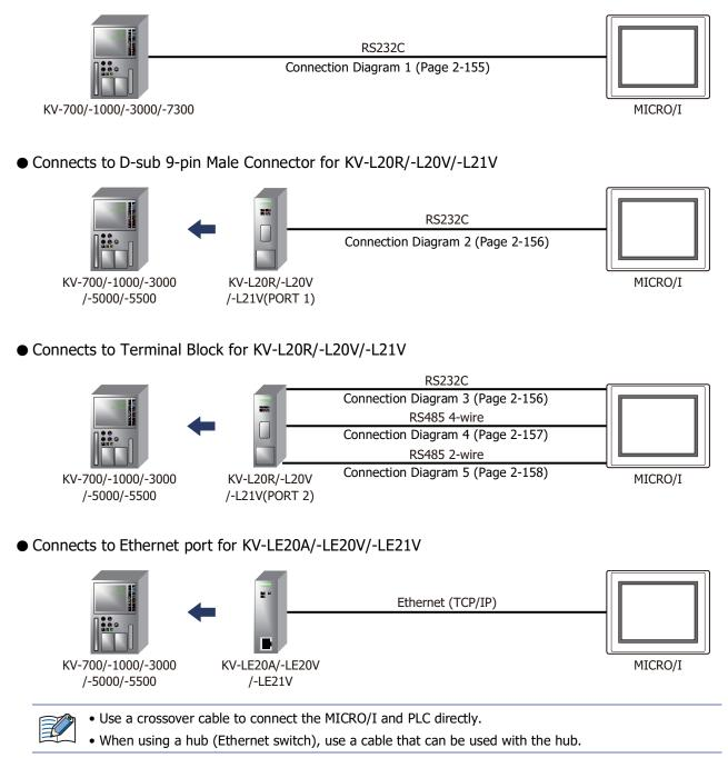
• Connects to Ethernet port for KV-5000/-5500/-7500
