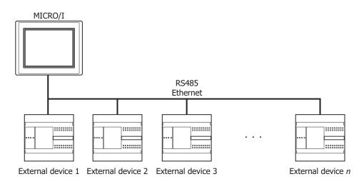
Different types of external devices can be simultaneously connected by using multiple communication drivers, refer to "5 Using Multiple Communication Drivers" on page 6-9.
