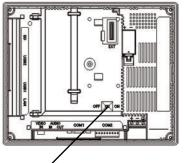
Terminating Resistor Selector Switch
