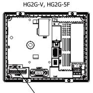
Terminating Resistor Selector Switch
