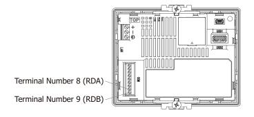
\*1 In case of the HG5G/4G/3G/2G-V, HG4G/3G, HG2G-5F inserts terminating resistor to only Terminal port, not D-sub port. Insert a terminating resistor (100 to 120 Ohm, 1/2 W minimum) when using RS422/485 interface at D-sub port if necessary.
