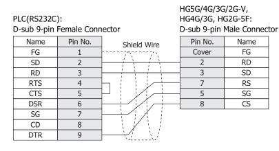
PLC(RS232C): D-sub 9-pin Female Connector
