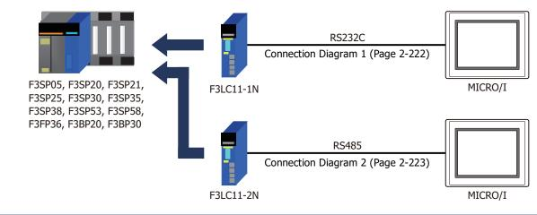
We recommend F3LC11-2N side to carry a "4-WIRE" setup of the terminus resistance (TERMINATOR) in long-distance transmission.
