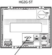
Terminating Resistor Selector Switch
