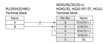
The HG4G/3G, HG2G-5F uses only RDA and RDB when using RS422/485 2-wire, therefore, you don't need to connect SDA or SDB.
