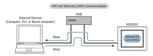
• The Event Transmission function cannot be used with DM Link Ethernet (UDP) communication.
