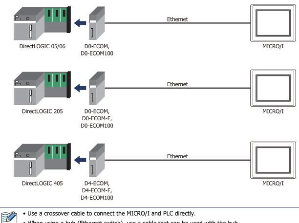
• When using a hub (Ethernet switch), use a cable that can be used with the hub.
