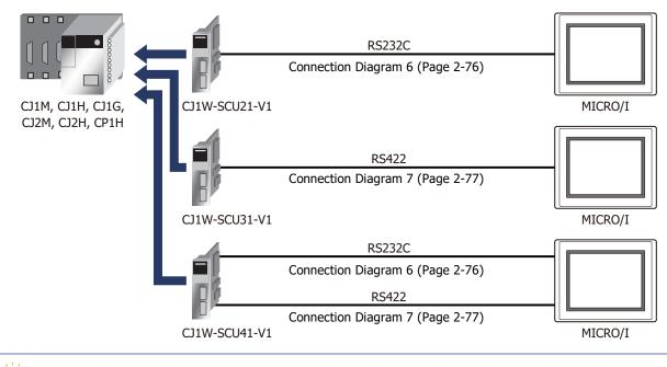
You can use the same cable for Connection Diagram 6 as for Connection Diagram 5.
