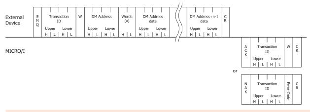
Do not transmit the following command until the external device receives the response of a command which transmitted to the display machine or serves as a timeout.
