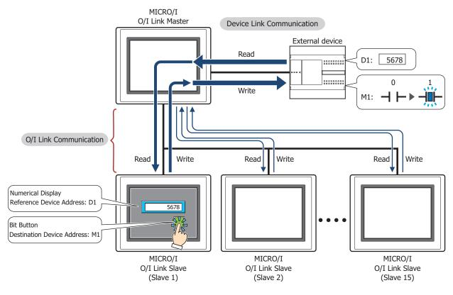
O/I Link Communication can only be used for the External Device Communication 1. The communication driver of O/I Link Slave should match the O/I Link Master's.
