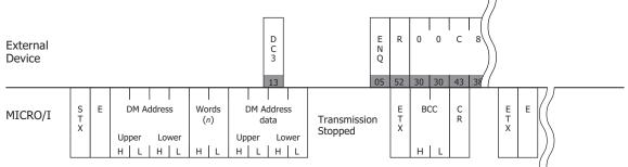
The shaded part of the command is ASCII code.
