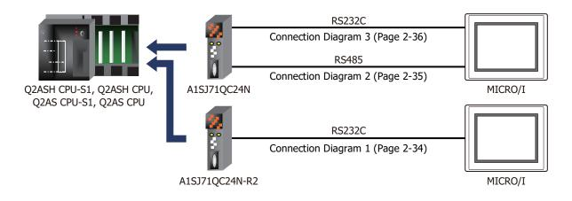
• MELSEC-Q Series (Connects to CPU Module Programming Port)
