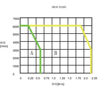
DM1 series servo motor T-N curves
