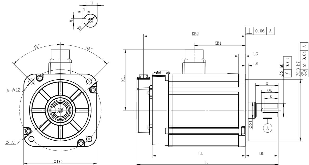
□ 130 flange motor dimensions (unit: mm)
