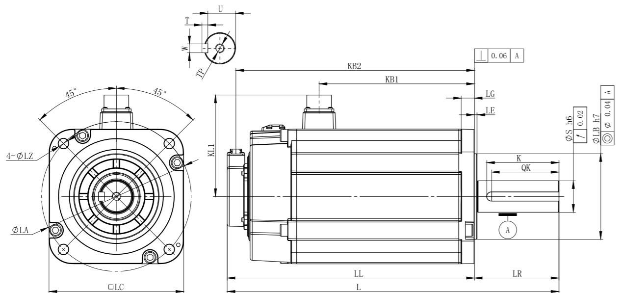
□ 180 flange motor dimensions (unit: mm)
