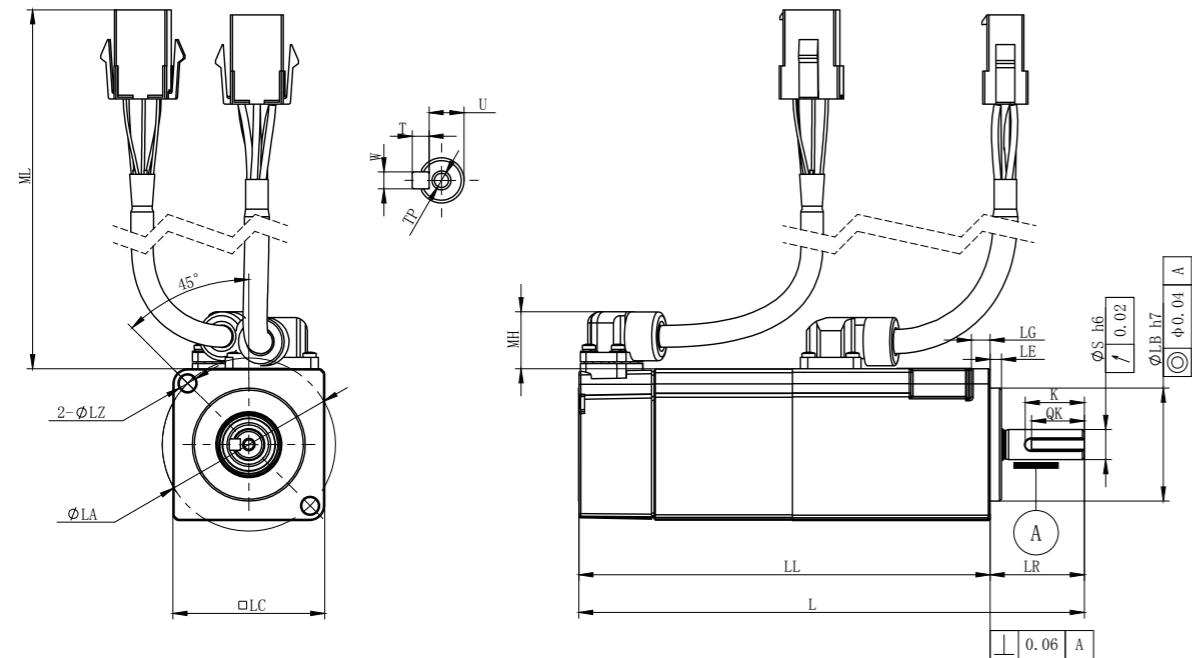
□ 40 flange motor dimensions (unit: mm)
