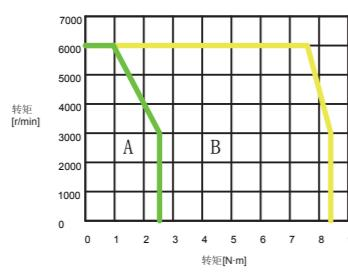
DM1 series servo motor T-N curves
