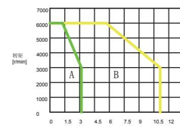
DM1 series servo motor T-N curves
