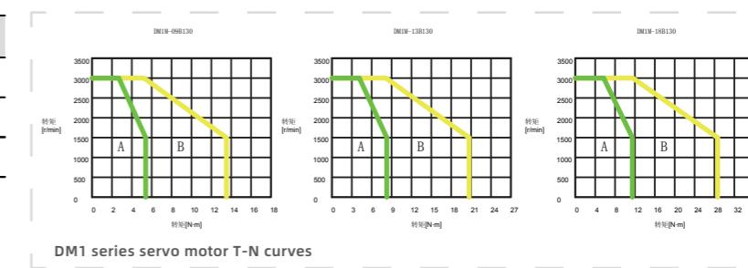
DM1 series servo motor T-N curves
