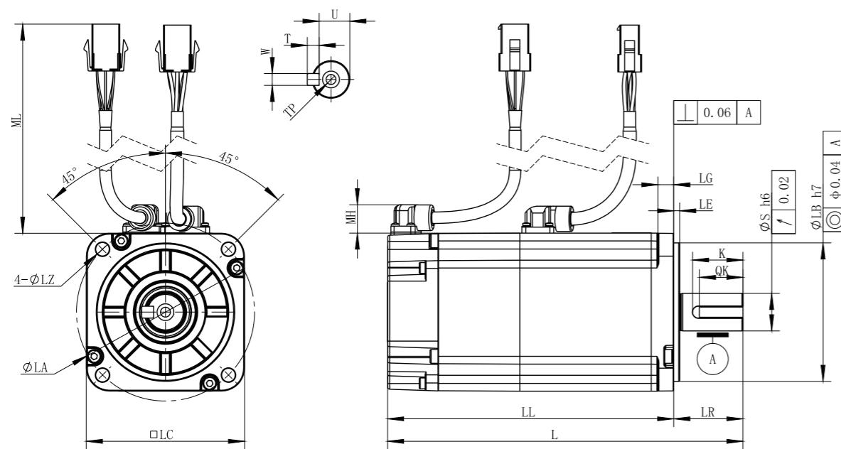
□ 80 flange motor dimensions (unit: mm)
