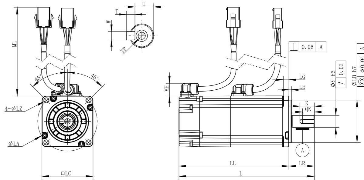
□ 60 flange motor dimensions (unit: mm)
