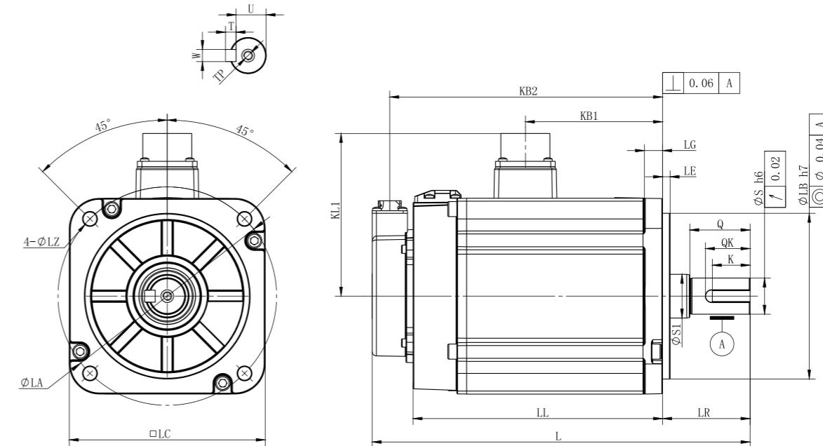
□ 130 flange motor dimensions (unit: mm)
