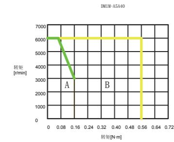
DM1 series servo motor T-N curves
