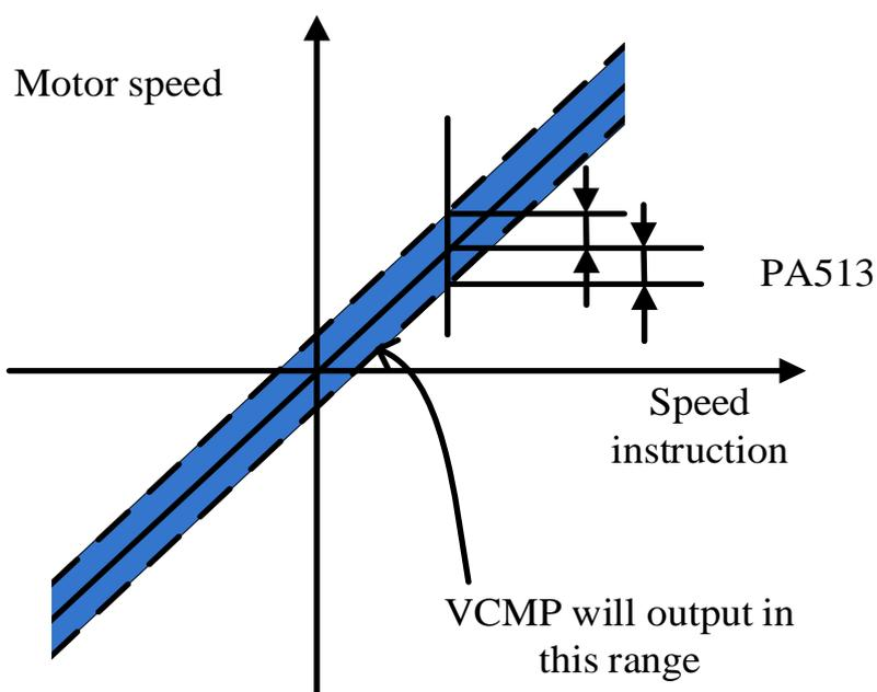
For example, PA513=100, speed instruction is 2000rpm, if motor speed is within 1900rpm to 2100rpm, VCMP will be ON.
