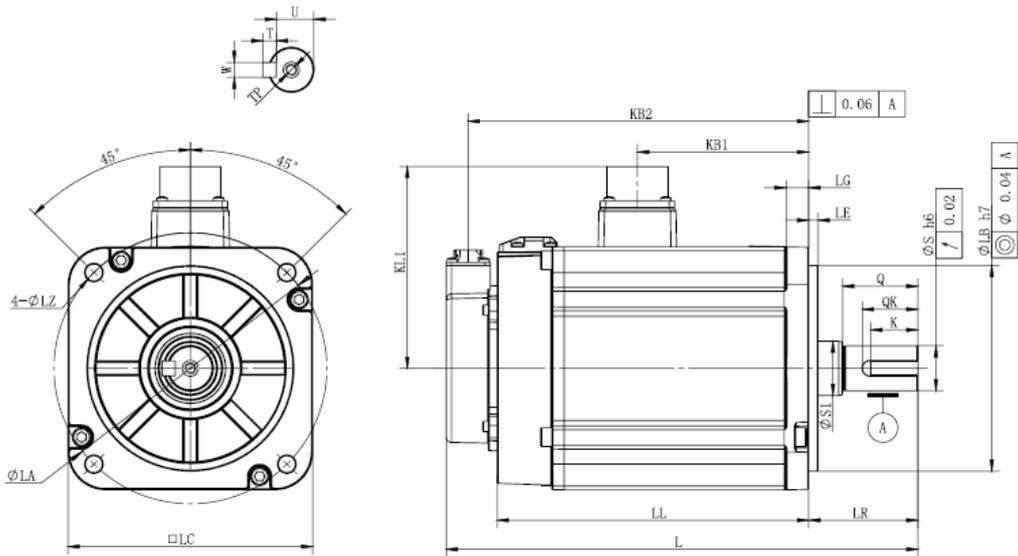
□130 flange motor dimensions (unit: mm)
