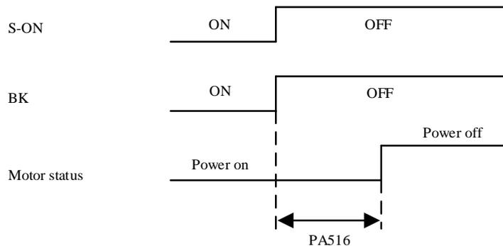
When an alarm is given out, the servo motor will be immediately powered off, and the setting of this parameter becomes irrelevant.
