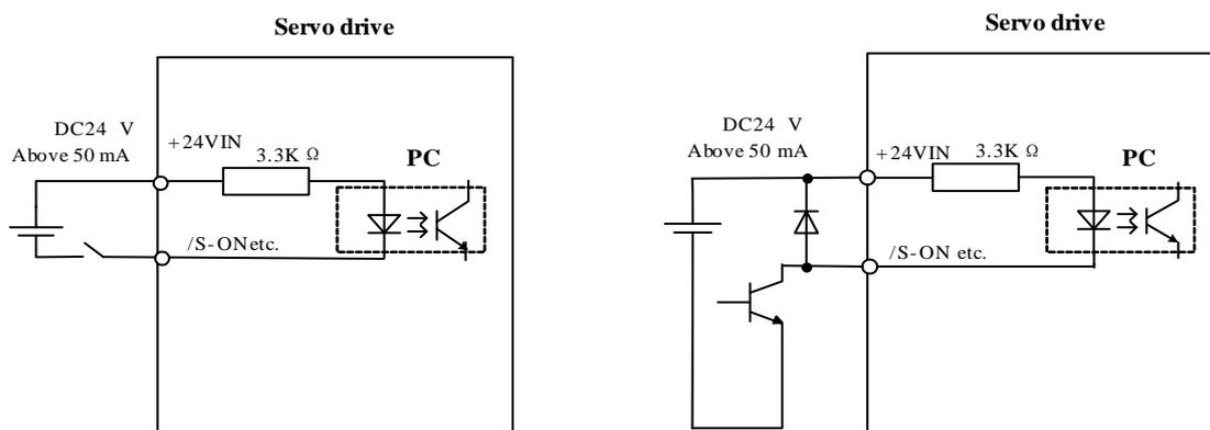
Take the above figure as an example. When the optocoupler is conductive, S-ON signal is L level; when the optocoupler is not conductive, S-ON signal is H level. Parameter PA500.2 decides the active level of S-ON. When PA500.0=2, S-ON signal is L level active; when PA500.2=1, S-ON signal is H level active.
