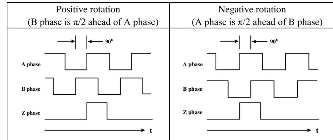
Please make servo drive rotate by two turns before using servo drive's Z phase pulse output for mechanical reference point reset action. If this can't be done due to the structure of the mechanical system, please implement reference point reset action at speed below 600rpm (calculated according to servo motor's rotating speed) .
