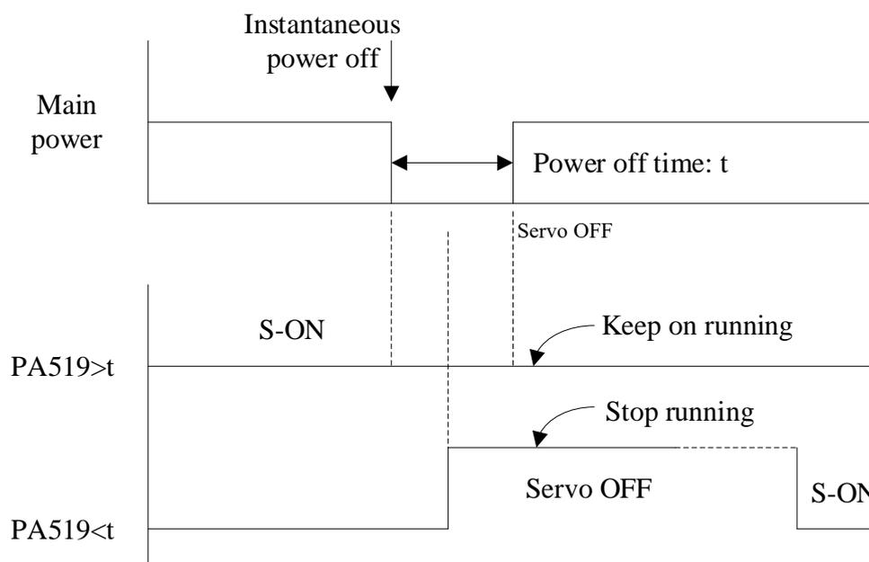
The maximum holding time setting value is 1000ms during instantaneous power off, but the holding time of control power supply of the servo motor is about 100ms. The holding time of main power supply varies along with the output of servo drive.
