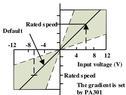
**Input voltage range:** DC  $\pm 2V \sim \pm 10V$  / rated speed
