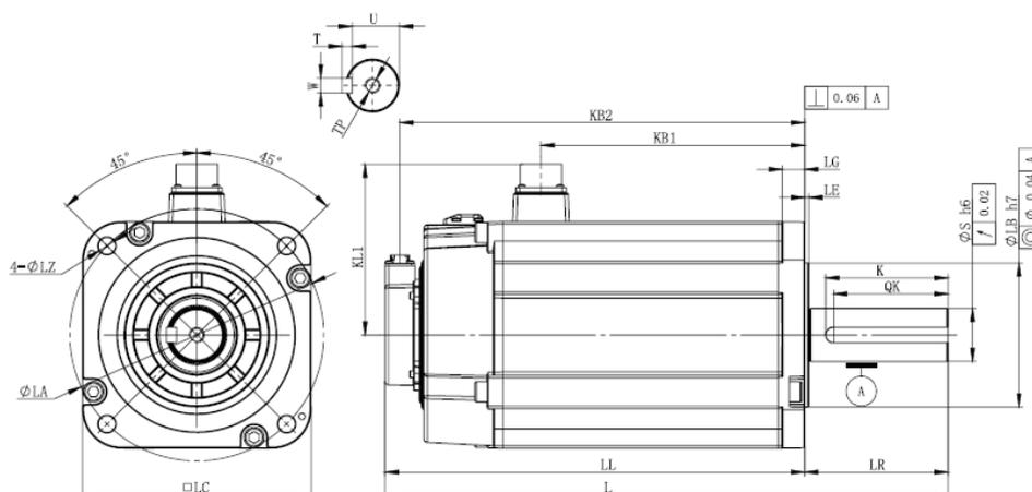
□180 flange motor dimensions (unit: mm)
