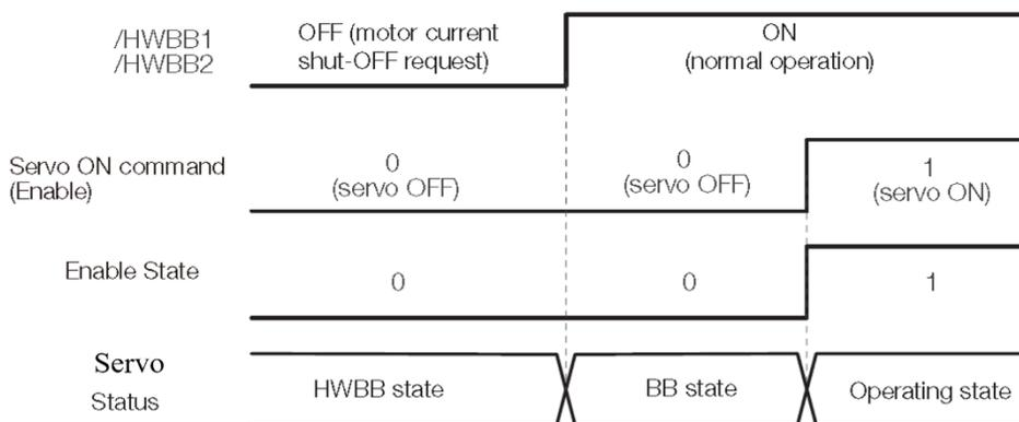
If the servo ON command is input while the / HWBB1, / HWBB2 signals are OFF, the HWBB status will remain unchanged even after the / HWBB1, / HWBB2 signals are turned ON.
