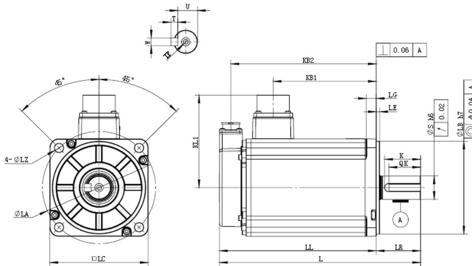
□100 flange motor dimensions (unit: mm)
