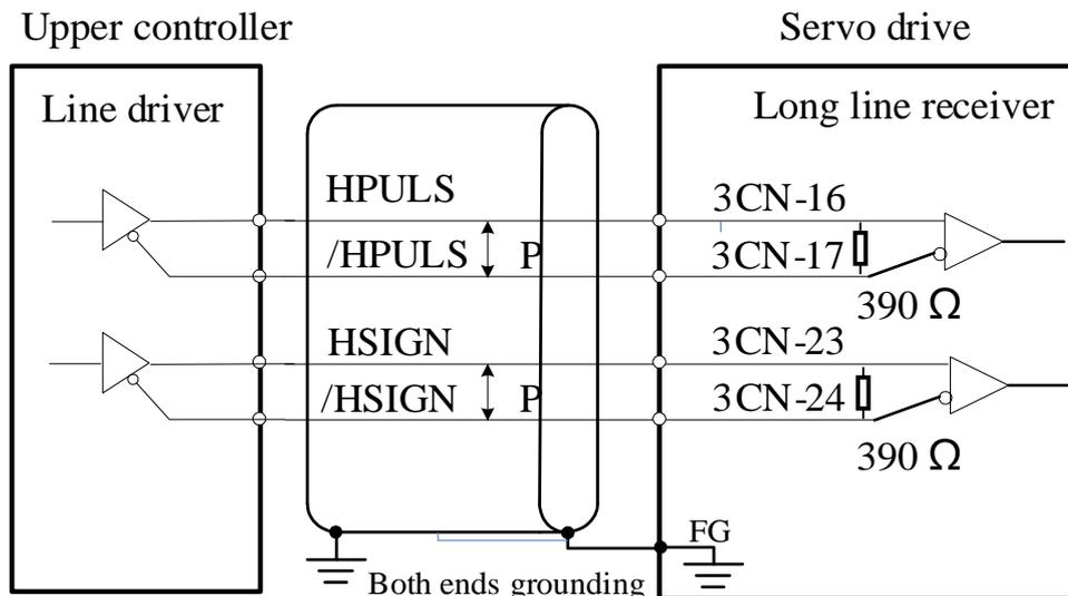
Compatible line driver: AM26LS31 (TI) or equivalent.
