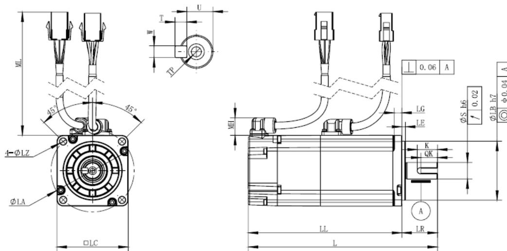
□60 flange motor dimensions (unit: mm)
