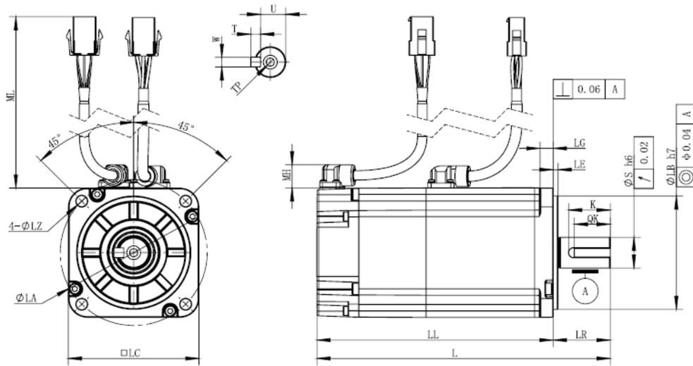
□80 flange motor dimensions (unit: mm)
