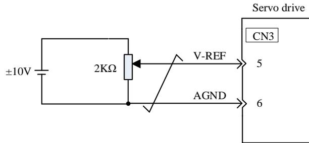
Programmable controller and so on are used for connection with the instruction controller's speed instruction output terminal in case of position control by
