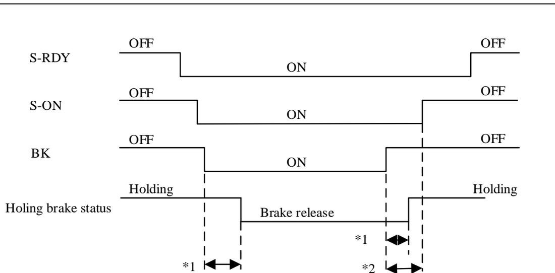
\*1. The time from BK signal active to brake release is different for different types of brakes.
