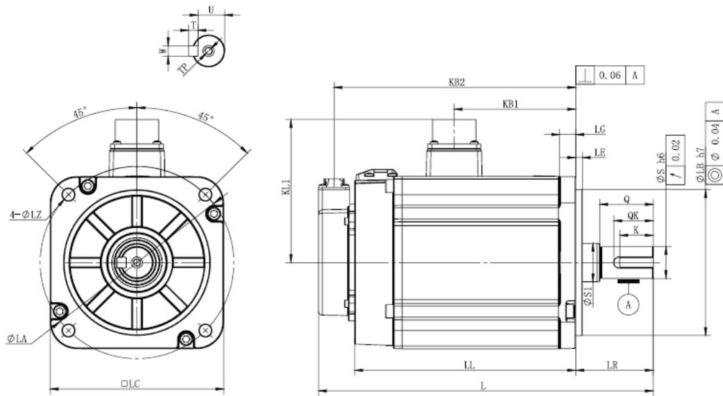
□130 flange motor dimensions (unit: mm)
